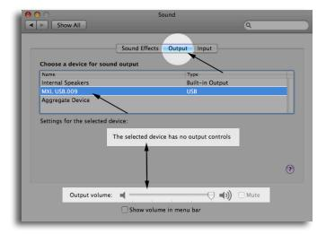
**5**. Further adjustments to the sample rate and bit-depths can be found in the **Audio Midi Setup** (Macintosh HD > Applications > Utilities > Audio Midi Setup.) You should however, check the settings in the recording program you are using as they may override or conflict with these settings.
